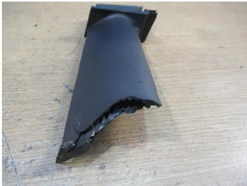
**Figure 2: Failed High Pressure Turbine Blade**
