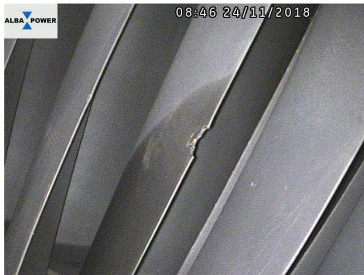
**Figure 3: Low Pressure Turbine Blade Impact Damage**
